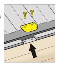
18. If installing struts for an extended top, remove the end caps from the front corners of the utility box.
