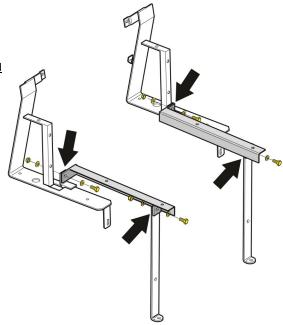
If reinstalling the OE top, loosely fasten the replacement rear struts to the front seat back supports using (4) M10 x 70 Hex Head Bolts,
