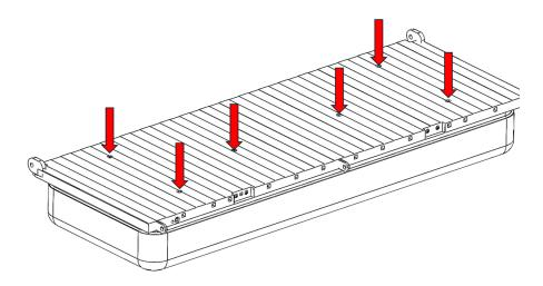
17. FOR SEAT-931 ONLY: Lock the seat bottom into place with the (2) small retaining plates and (4) M6 x 15 Phillips Head Countersunk Screws (Bag #5).
