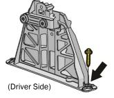
Remove the (2) bolts at the top of the bagwell area. Retain hardware.
